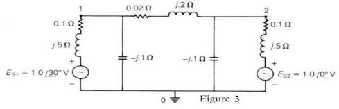
Determine the  $4 \times 4$  bus admittance matrix  $Y_{\text{bus}}$  and write nodal equations in matrix format for the circuit shown in Figure 3. Do not solve
